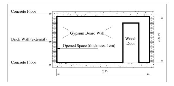
Figure 5: Schematic gypsum board partition with gaps represented in bold lines.
